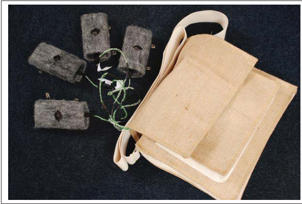
Figure 2. Spatial Density sensors and shoulder bag
