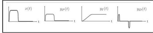
**Figure 2.** Functional transformation produced by proportional, integral and differential operators to a smoothed and large pulse  $x(t)$  as input function.
