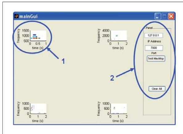
**Figure 4.** Matlab GUI. Spike representation of four sounds (sonic landmarks) representative of the entire sound space generated by means of the SDT friction model. By clicking in the graphical area around a spike representation it is possible to listen to the corresponding sound (see the area highlighted by circle 1). Circle 2 shows the control panel for the communication with the SDT model in Max/MSP
