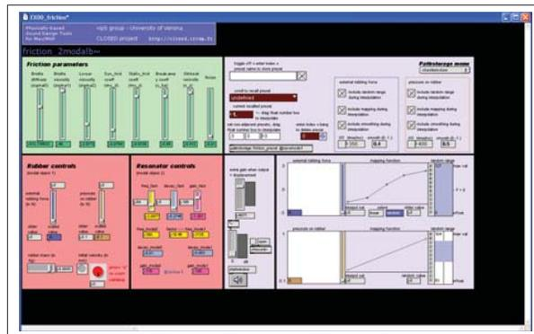
**Figure 1.** The friction MAX/Pd patch, contained in the SDT synthesis tools package. The user can tune up to 27 synthesis parameters representing the driving forces, the characteristics of the modal resonators, and the characteristics of the nonlinear interaction.
